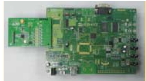
GCT Bluetooth Evaluation Board Kit (EBK)
